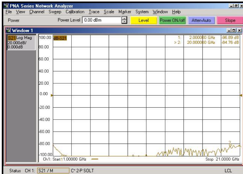
Figure 15 Typical On/Off Ratio of the PIN Switch
